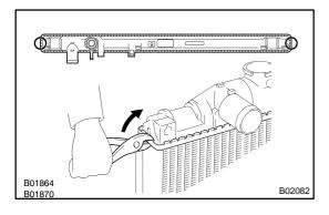
The points shown in the illustration cannot be staked with the SST. Use pliers or similar object and be careful not to damage the core plates.
