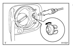
(b) Rotate the retainer to the left to disengage the lock, then pull it out.
