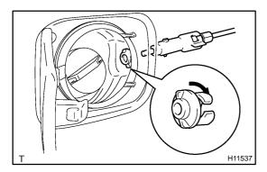
(b) Insert the fuel lid lock control to the retainer and rotate it to the left to lock.
