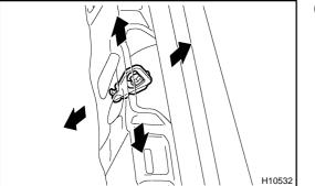
(c) Using a hammer and brass bar, tap the striker to adjust it. **Torque: 5.5 N·m (56 kgf·cm, 49 in.·Ibf)**
