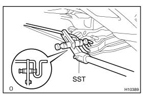
(b) Install SST to the torsion bar on the hinge side. SST 09804-24010
