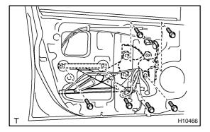
(a) Install the window regulator with the 6 bolts.
