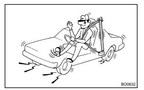
(b) Drive the car at 10 mph (16 km/h) and slam on the brakes. Check that the belt locks and cannot be extended at this time.
