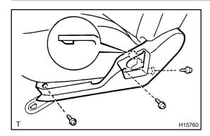
INSTALL FRONT SEAT CUSHION OUTER SHIELD Install the front seat cushion outer shield with the 3 screws.
