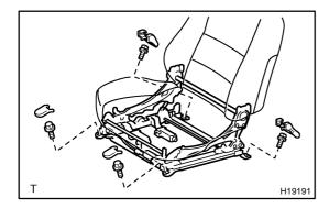
(d) Temporarily tighten the bolts on the front side. Then, tighten them to the final torque starting from the inner side.
