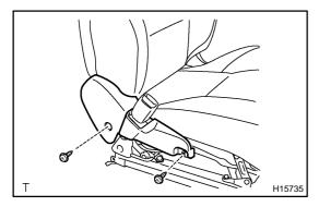
**13. INSTALL FRONT SEAT CUSHION INNER SHIELD** Install the front seat cushion inner shield with the 2 screws.
