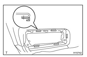
(h) Slide the airbag door downward to install it.
