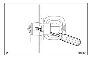
(b) Using a screwdriver, disengage the claw on the accessory ry socket cover from the body and remove the accessory socket and cover as a unit.
