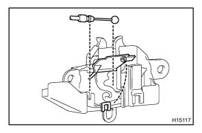
(c) Using a screwdriver, open the cover, then disconnect the hood lock control cable.
