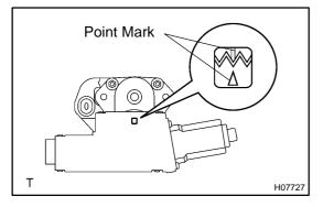
(c) Turn the drive gear to align the point marks as shown in the illustration.
