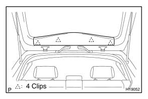
**16. INSTALL BACK DOOR TRIM BOARD UPPER** Install the back door trim board upper to the body.
