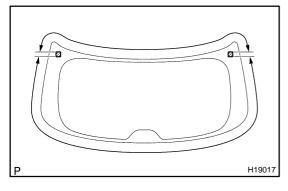
e) Let the piano wire pass as shown in the illustration, cut off the adhered part to the clips.
