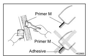
8. COAT CONTACT SURFACE OF BODY WITH PRIMER "M"
