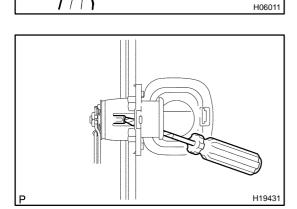
(b) Using a screwdriver, disengage the claw on the accessory socket cover from the body and remove the accessory socket and cover as a unit.
