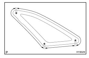
(e) Cut the adhesive by pulling the piano wire around it. HINT:
