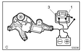
(b) Disconnect the negative (-) lead from terminal 1, check that the motor stops running at the stop position.If operation is not as specified, replace the motor.
