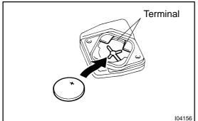
(e) Install a battery (lithium battery) as shown in the illustration.
