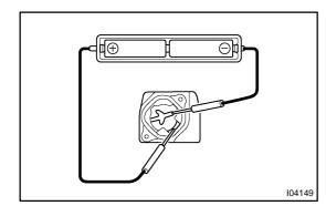
(c) Install a new or normal battery (lithium battery). HINT:
