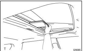
(b) When the tilt-down operation is being used: Check that the sliding roof fully tilts up when an object is caught between the vehicle body and the roof glass.
