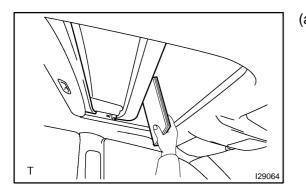
(a) When sliding roof AUTO operation is being used: check that the roof glass should open a distance of 200 mm (7.87 in.) from the point of contact with the object, or fully open if 200 mm (7.87 in.) of opening distance is not available when an object is caught between the vehicle body and the roof glass.
