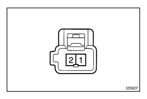
5. INSPECT SEAT CUSHION FRONT SIDE CONTINUITY Inspect the seat cushion front side continuity between terminals, as shown.
