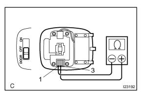
(c) Turn the room light switch DOOR, check that continuity exists between terminals 1 and 3.
