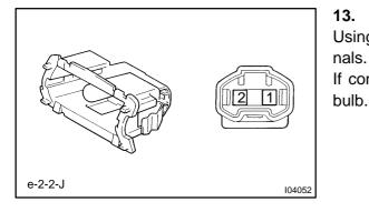
**13. INSPECT DOOR COURTESY LIGHT CONTINUITY** Using an ohmmeter, check that continuity exists between termi-
