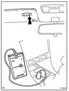
(b) Press the switch which an inspection code has been registered for and check that LED (green) of the home link tester lights up.
