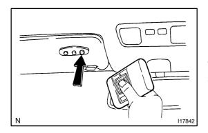
(b) In the condition of (a), bring the original transmitter to within 1-inch area around the garage door opener and press the switch. (code transmitting).
