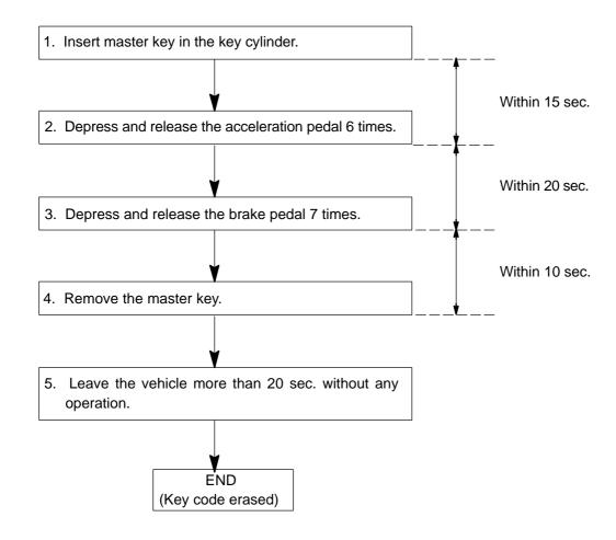
(1) Depressing brake pedal and acceleration pedal:
