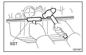
(b) Install the blade of SST between the transmission case and oil pan, cut off applied sealer, and remove the oil pan. SST 09032-00100
