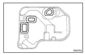
(b) Remove the 3 gaskets from the oil strainer.
