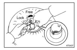
(b) Press on the serrations of starter with a finger and rotate it.
