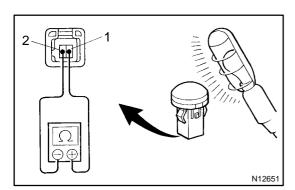
(b) Remove the cloth from the sensor and subject the sensor to electric light, check that continuity exists between terminals.
