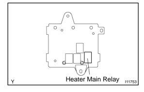
(c) Remove the heater main relay from passenger side junction block.
