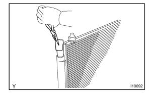
(c) Using pliers, remove the dryer.
