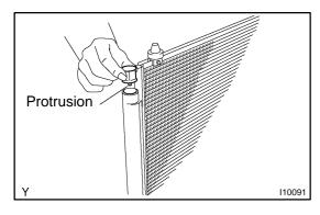
(e) Insert the filter into the modulator.
