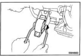
(c) Remove the front mounting bolt and mounting.
