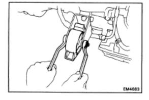
(b) Install and torque the front mounting bolt.
