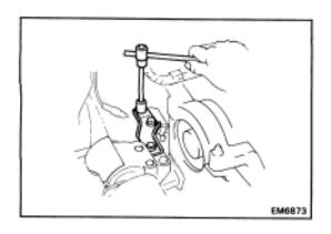
(g) Install the RH mounting stay with the three bolts.
