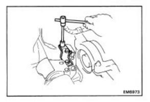
(b) Remove the three bolts and mounting stay.
