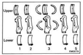
HINT: Arrange the main bearing caps, bearings and thrust washers in correct order.
