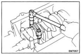
(b) Remove the connecting rod cap nuts.
