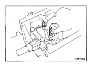
(d) Cover the connecting rod bolts with a short piece of hose to protect the crankshaft from damage.
