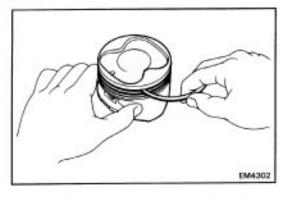
(b) Using a groove cleaning tool or broken ring, clean the piston ring grooves.
