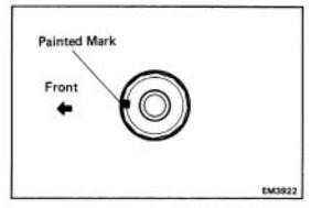
(e) Mark the front side of the top of cap nut with paint.
