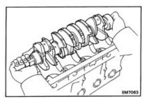
(c) Lift out the crankshaft.
