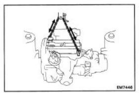
(d) Install the RH mounting insulator to the engine mounting bracket with the two nuts.
