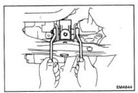
(d) Remove the rear mounting bolt and mounting.
