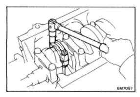
(i) Remove the connecting rod cap. (See procedure (b) and (c) on page EM-132.)
