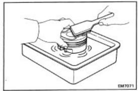
(c) Using solvent and a brush, thoroughly clean the piston. **NOTICE: Do not use a wire brush.**
