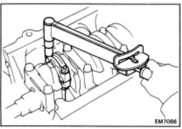
(h) Install the connecting rod cap.(See step 7 on page EM-154)NOTICE: Do not turn the crankshaft.
