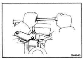
(i) Install the PS pump pipe clamp bolt.
