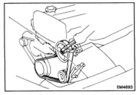
(g) Tighten the PS pump pulley nut. **Torque: 390 kg-cm (28 ft-lb, 38 N-m)** (h) Connect the two A/C connectors.
