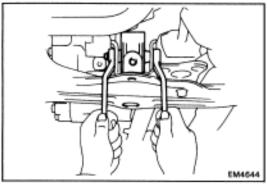
(f) Install and torque the front mounting bolt.
