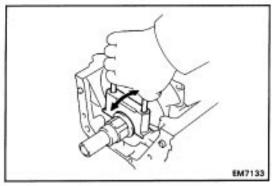
(b) Using the removed main bearing cap bolts, pry the main bearing cap back and forth, and remove the main bearing caps, lower bearings and lower thrust washers (No.3 main bearing cap only).
