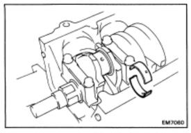
(e) Clean the crank pin and bearing.
