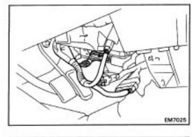
(f) Pull out the engine wire from the cowl panel.
