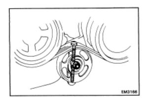
(f) Install the drive belt, and temporarily tighten the idler pulley bolt.
