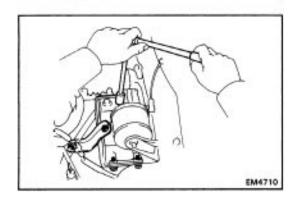
(d) Install the RH mounting insulator to the engine mounting bracket with the two nuts and bolt.
