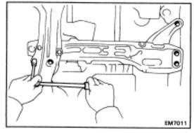
(c) Install the engine mounting member with the five bolts. Torque the bolts.
