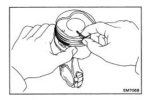
(b) Remove the two side rails and oil ring expander by hand. HINT: Arrange the rings in correct order only.
