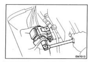
(b) Remove the two nuts, through bolt and RH mounting.
