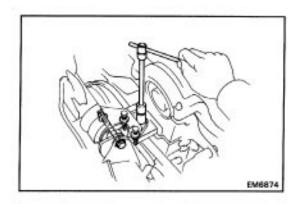
(c) Remove the bolt, two nuts, through bolt and RH mounting.
