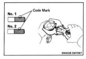
(b) Using a piston ring expander, install the two compression rings with the code mark facing upward.
