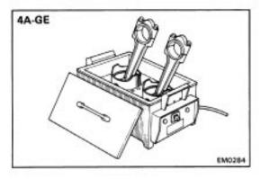
(b) Gradually heat the piston to  $70 - 80^{\circ}$ C (158 – 176°F).
