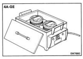
(b) Gradually heat the piston to  $70 - 80^{\circ}$ C (158 – 176°F)
