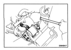
(f) Align the LH mounting insulator bracket with the transaxle case bracket. Temporarily install the three bracket bolts.
