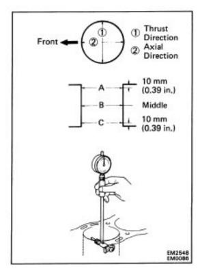
Using a cylinder gauge, measure the cylinder bore diameter at positions A, B and C in the thrust and axial directions.
