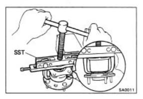
2. REMOVE AXLE SHAFT FROM AXLE HUB
