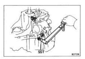
(b) Apply sealant to the plugs and lock ball assembly threads. Sealant: Part No.08833-00080, THREE BOND 1344,
