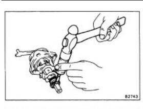
(j) Install the compression spring, seat and E-ring.
