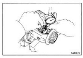
(d) Measure the side gear backlash while holding one pinion gear toward the case.
