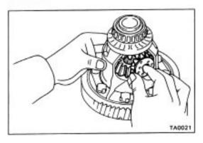
(c) Remove the two pinion gears and two side gears with the four thrust washers from the case.
