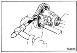
(i) Using a hammer and drift punch, stake the locking plates. HINT: Stake one claw flush with the flat surface of the nut. For the claw contacting the protruding portion of the nut, stake only the half on the tightening side.
