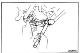
(b) Using a plastic hammer, carefully tap the oil pump body.
