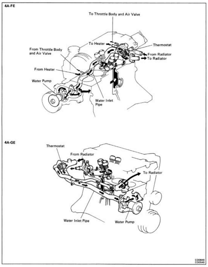
The cooling system is composed of the water jacket (inside the cylinder block and cylinder head), radiator, water pump, thermostat, electric fan, hoses and other components.
